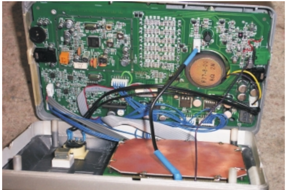
Blick in das Innere des DRM-Receivers 2010 von Mayah Communications
